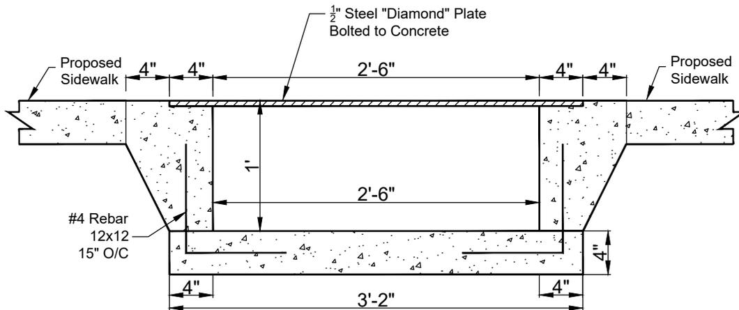
1. Concrete Sidewalk Shall Be Formed With 4" Forms, And Not Earth Formed.
